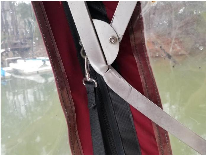
Unfortunately, our sole physical asset, the Committee Boat, suffered damage during a storm this past month. We are not sure which storm, but one of them resulted in the canvas enclosure collapsing with broken support rods. The collapse also resulted in some ripped fabric.
